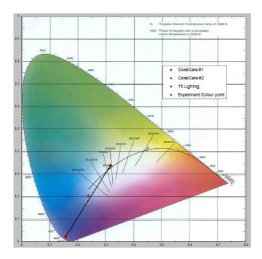
Figure 3: CIE 1931 xy chromaticity space of both light sources, with T5 represented by a purple diamond, and the CoralCare LED by red diamonds. The red diamond in the middle of the black line, close to the purple T5 diamond, represents the LED colour point used in this experiment.
