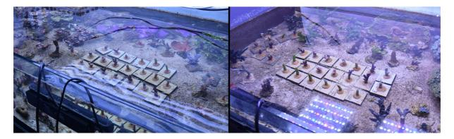
Figure 5: In both sections of the setup, corals were placed randomly and rotated weekly within their group to cancel out local variations in irradiance, spectrum and water flow rate. Left: T5, right: LED.
