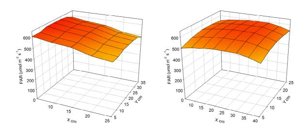
Figure 2: PAR landscape of the T5 luminaires (left) and the CoralCare LED units (right) as seen from the front of the experimental setup. Mean PAR values of the T5 luminaires and CoralCare LED units were  $561\pm42$  S.D. and  $565\pm29$  S.D.  $\mu$ mol  $m^{-2}$   $s^{-1}$ , respectively. Only the areas in which the corals were placed are plotted. Note that corals within both treatments were randomly rotated weekly to cancel out local PAR variations.
