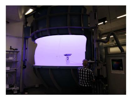
Figure 4: The optical measurement sphere at Philips, used to determine the wall–plug efficiency of both light sources. Only the CoralCare LED unit is shown here. During measurements, the sphere is completely closed to measure all light emitted by the source.
