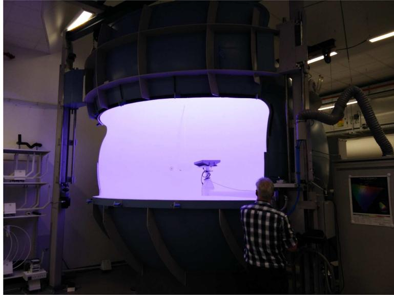
*Figure 4: The optical measurement sphere at Philips, used to determine the wall-plug efficiency of both light sources. Only the CoralCare LED unit is shown here. During measurements, the sphere is completely closed to measure all light emitted by the source.*
