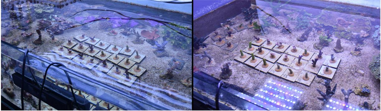
Figure 5: In both sections of the setup, corals were placed randomly and rotated weekly within their group to cancel out local variations in irradiance, spectrum and water flow rate. Left: T5, right: LED.
