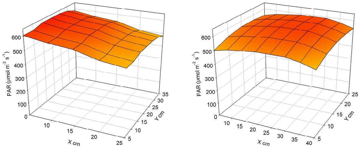
*Figure 2: PAR landscape of the T5 luminaires (left) and the CoralCare LED units (right) as seen from the front of the experimental setup. Mean PAR values of the T5 luminaires and CoralCare LED units were  $561 \pm 42$  S.D. and  $565 \pm 29$  S.D.  $\mu\text{mol m}^{-2} \text{s}^{-1}$ , respectively. Only the areas in which the corals were placed are plotted. Note that corals within both treatments were randomly rotated weekly to cancel out local PAR variations.*
